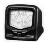
The SX20C is a compact SWR-power meter. Featuring cross needle design for measuring SWR and output power simultaneously. Compact size makes it very useful for testing mobiles as well as base station installation.
