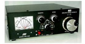
The world's only 300 Watt AirCore<sup>™</sup> Roller Inductor Tuner. Get your SWR down to absolute minimum -- something a tapped inductor tuner just can't do. Continuous coverage 6 Meters thru 160 Meters.
