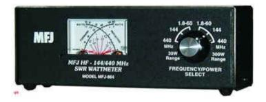
The **MFJ-864** cross-needle meter reads forward and reflected power and SWR simultaneously at a single glance. It features separate HF and VHF/UHF directional couplers, each with its own SO-239 connectors. This lets you connect your HF and VHF/UHF transceivers at the same time. You can then monitor SWR and power of either transceiver at the flick of switch. Others have a single set of connectors -- you have to plug and unplug to use separate HF or VHF rigs.
