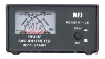
The **MFJ-860** cross-needle meter reads forward and reflected power and SWR simultaneously at a single glance. This meter may be used for 1.8 to 60 MHz up to 300 watts. The two power ranges are selected by a push button: 30/300 watts forward (and 6/60 watts reflected). The rear has SO-239 jacks for input and output. Meter uses 12 VDC.
